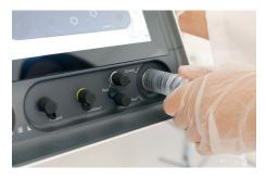
Canopy tests require a simple set-up by connecting the canopy hose to the blower
